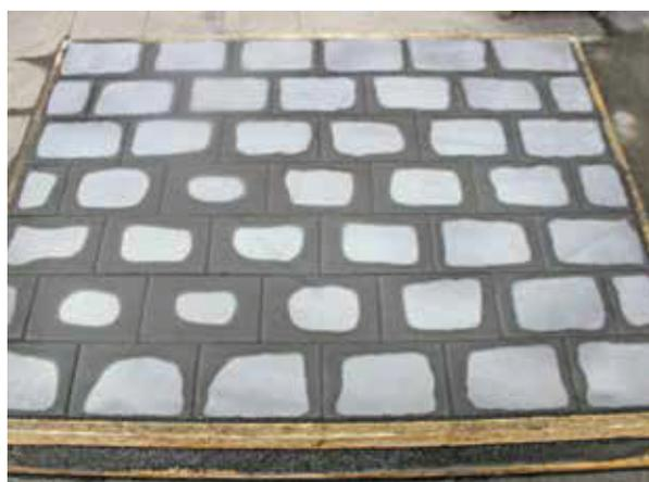
**Fig. 14a:** Prolonged drying of pavers ...
