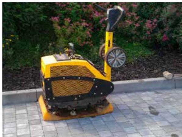
Fig. 16: Use of a paving pad
